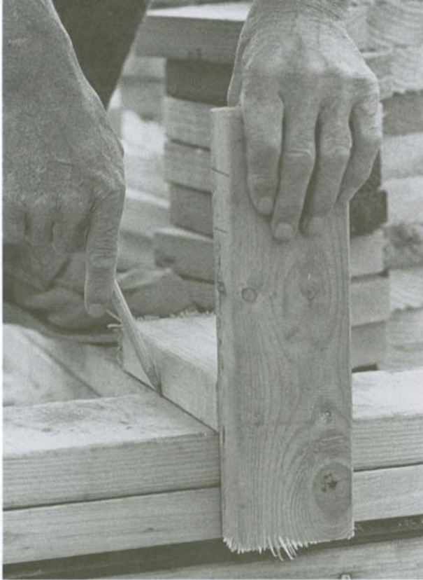
A channel marker allows for quick and accurate detailing of corners and channels.
